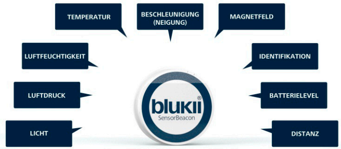
Industry 4.0: Sensor beacons are suitable for cost-efficient data capture (Source: www.blukii.com)
