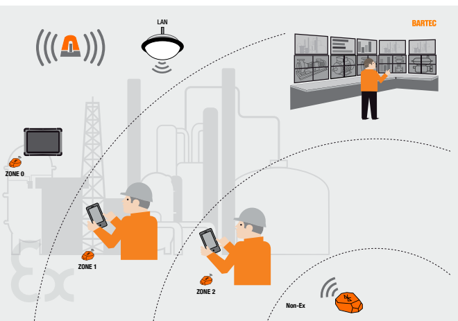
Access control: When a mobile device detects the beacon signal, checks using WLAN in the back-end establish whether the mobile device or its wearer are permitted to be in the respective potentially explosive atmosphere.
