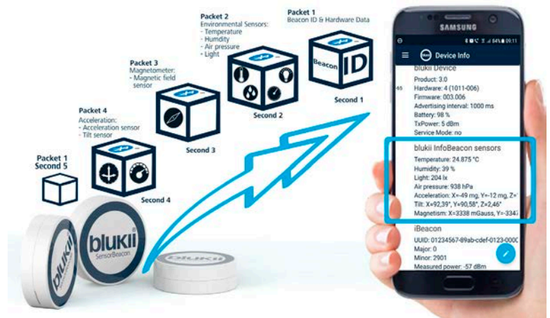
Industry 4.0: Sensor beacons transmit all measurement data packages at an adjustable advertising interval. (Source: www.blukii.com)
