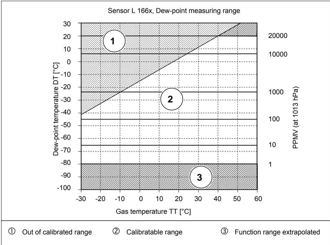
The sensor L 166x has a calibrated measurement range of -80 ° C ... +20 ° C DT in the pressure range up to 100 bar (200 bar per test certificate). The sensor measures with an accuracy of  $\pm 1$  K.
