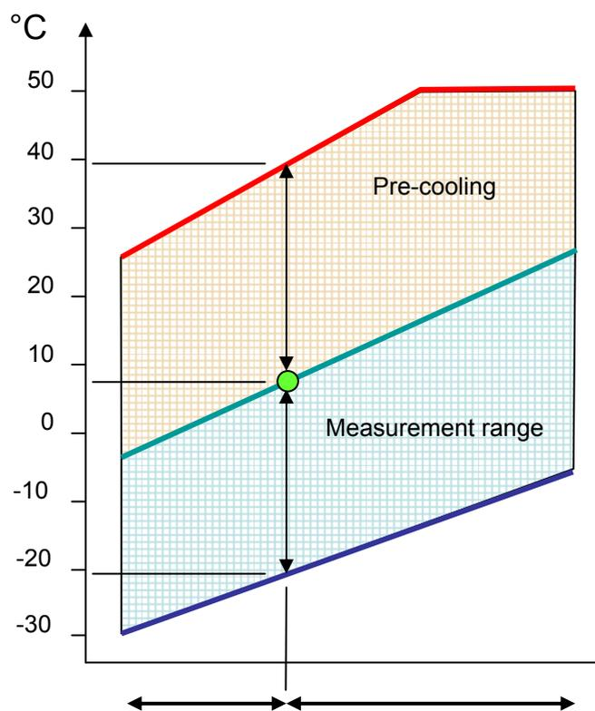
By default setting pre-selected sensor shaft temperature determines the dewpoint measurement range
