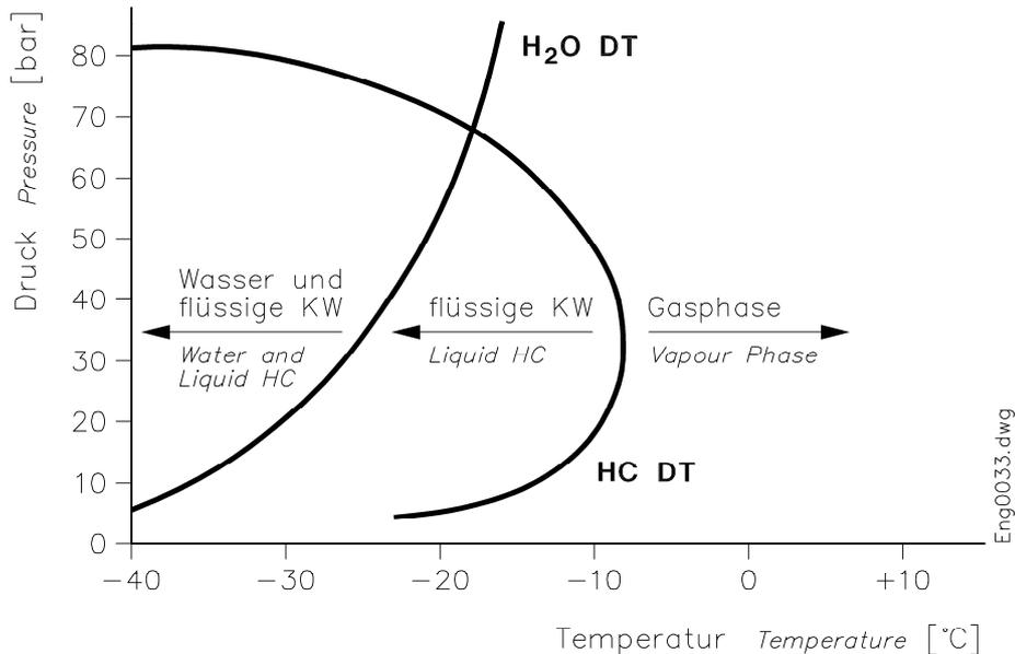
As can be seen in Fig. 1, in most of the cases the higher hydrocarbons condense before the water. The phase diagram (HCDT curve in Fig. 1) can be calculated from the composition of the natural gas. Fig. 2 shows an exemplary phase diagram. The condensation curve represented there contains two extremums: the cricondentherm point and the cricondenbar point.
