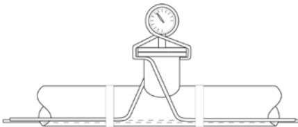
Installation on pressure gauges
