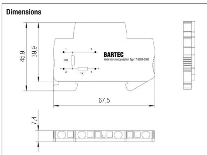
The resistive coupling element is used to monitor open and short circuits in isolator amplifier circuits controlled by mechanical contacts. The coupling element is installed directly to the control contact or inside its terminal box.
