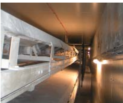
Graphic 4: Installation of the RedGuard® sensor cable on the upper side in the centre of a conveyor belt.
