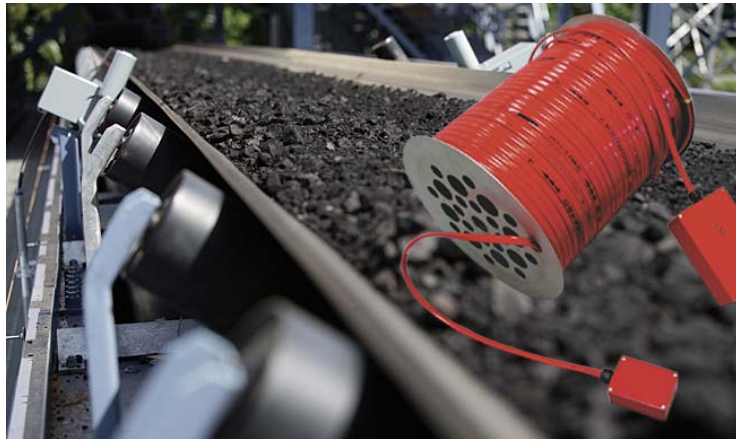
Graphic 1: Frictional heat of the belt, malfunction of bearings of rollers, coal which fell over a belt can cause a fire. The RedGuard® system offers an optimal monitoring solution.
