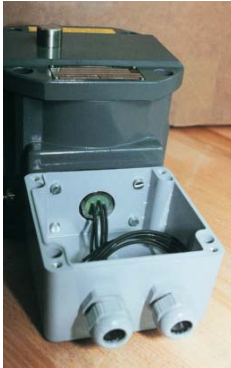
Line bushings in the Ex e terminal box
